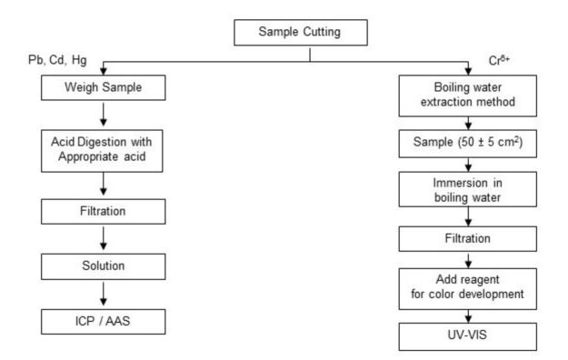
The metallic samples were dissolved totally by pre-conditioning method according to above flow chart for Cd, Pb and Hg contents analysis.
